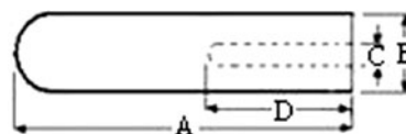
Fig. 4 Dilatometry test specimen ( A = 50 , B = 10 , C = 5 , and D = 25 ). All dimensions are in mm
